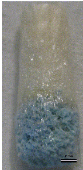
Figure 1-3. Chitosan/HAp bilayered scaffold showing two different layers, respectively for cartilage (upper layer) and bone (bottom layer). Reprinted with permission [49]. Copyright 2006, Elsevier.
