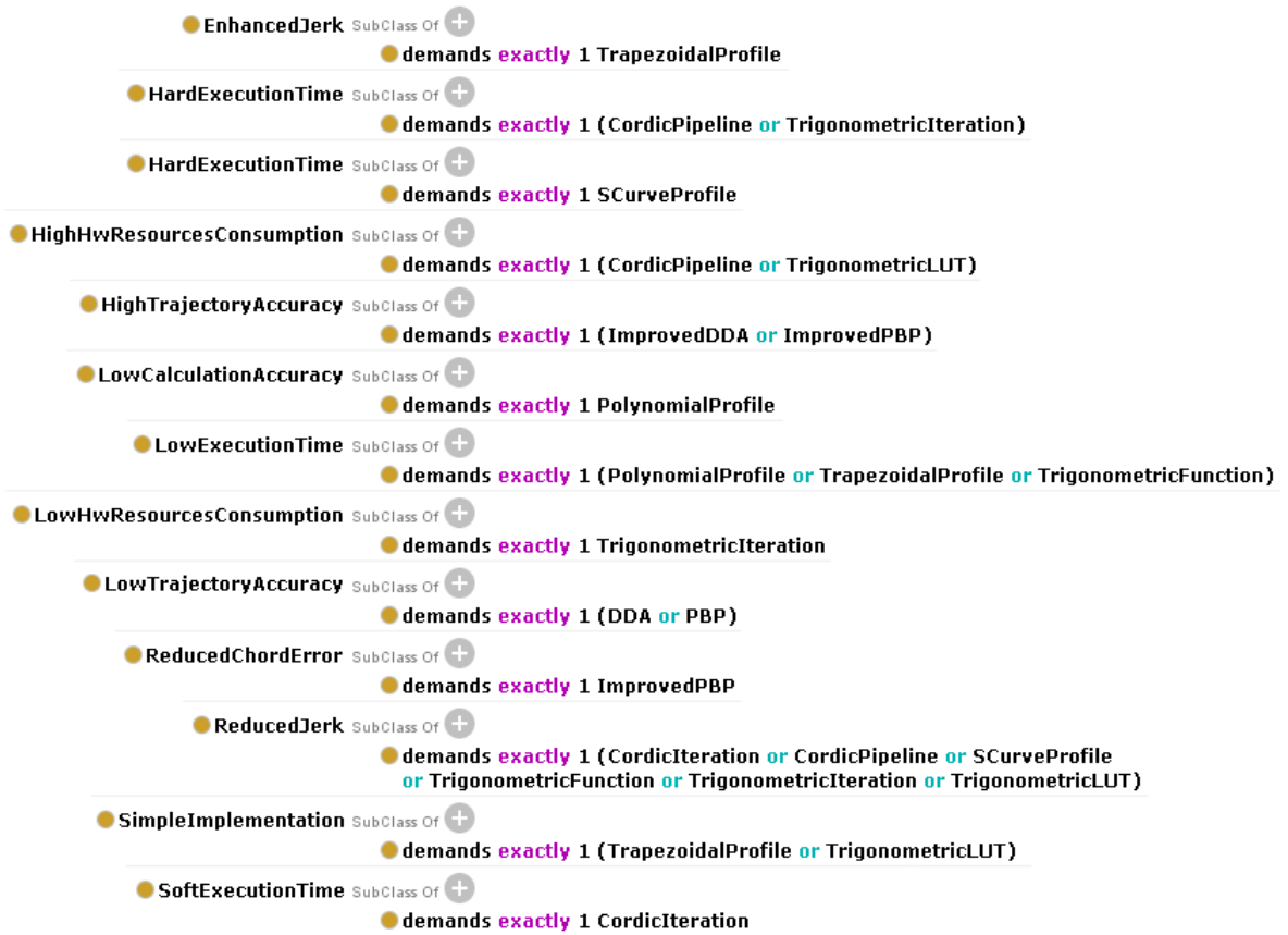
Figure 81.: Relation between processes and features of the coil winding machine (adapted from Prétége).
