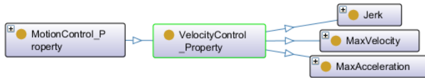
Figure 78.: Properties of a velocity control algorithm that has direct influence in system’s variability.
