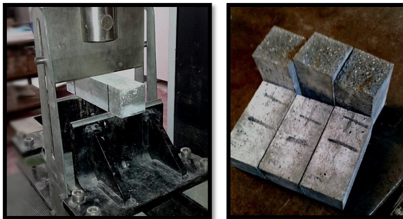
Figure 4-1 The three-point flexural test machine
