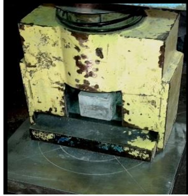
Figure 4-2 The compressive machine with a sample under distributed pressure.
