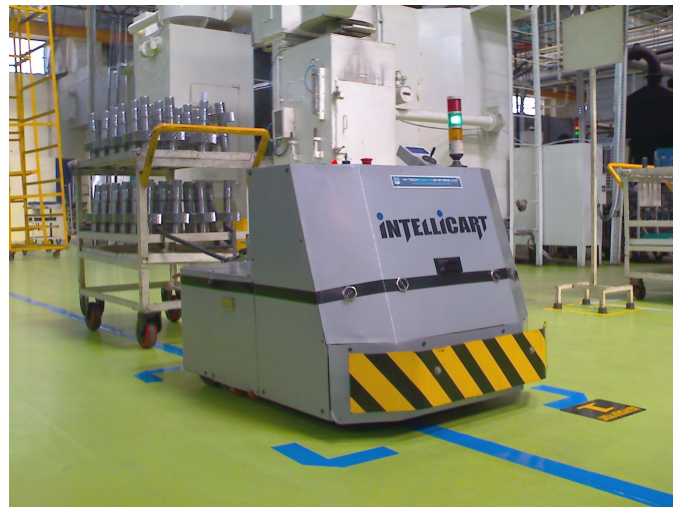
Figure 1.1: The Tow Type AGV following a predefined blue path (Mukeshhrs, 2009).
