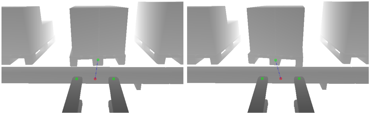
Figure 7.2: Detection results for a pallet with 4.7^\circ (left) and -8.0^\circ (right) orientation displacement.
