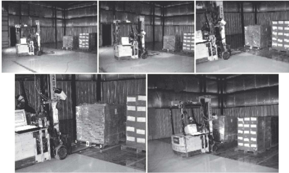
Figure 2.5: Prototype forklift engaging a pallet during experimental tests (Seelinger and Yoder, 2006).
