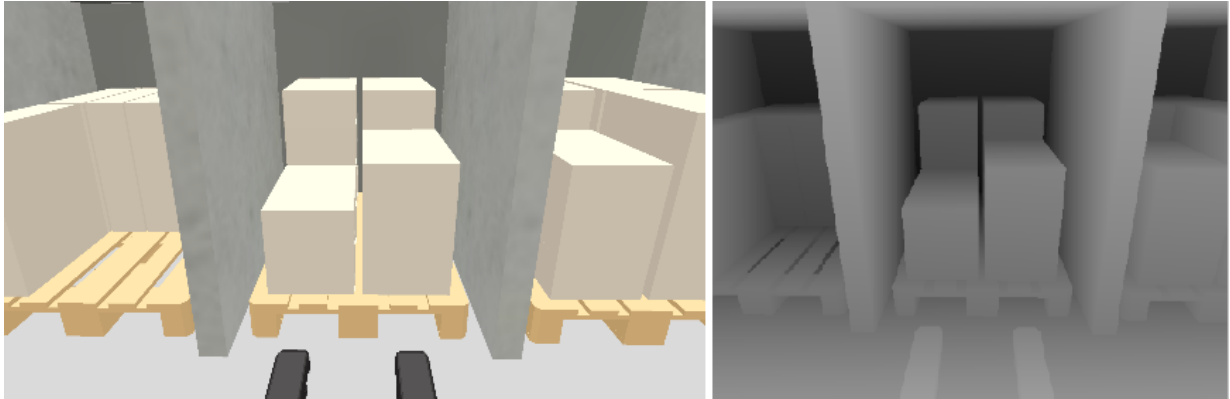
Figure 5.11: Pallet seen from the Intel RealSense inside V-REP simulator. At left the RGB image and on the right the depth image (RGB-D) resultant from the vision sensor.
