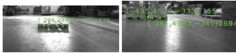
Figure 2.6: Successful detections in difficult cases. 3D point and orientation angle is indicated for each pallet (Varga and Nedevschi, 2014).
