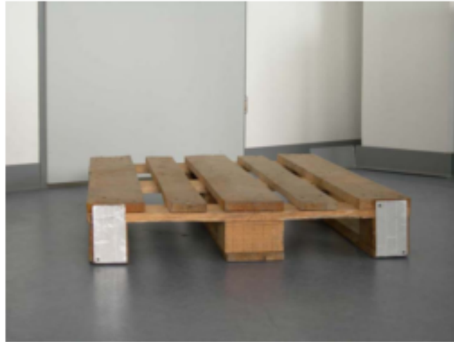
Figure 2.3: Euro pallet modified with reflectors (Lecking et al., 2006).
