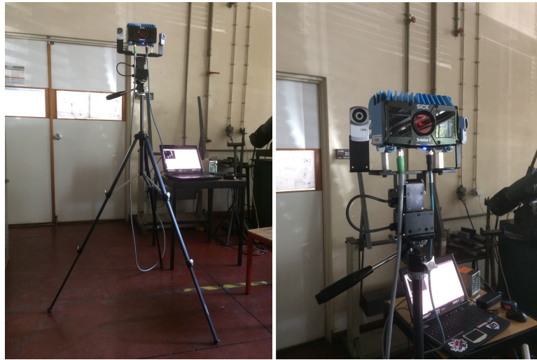
Figure 7.3: Testing bench created to simulate a real scenario for pallet detection.
