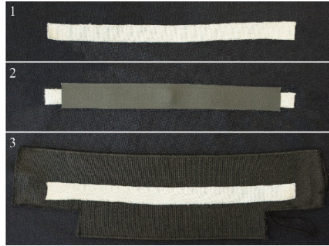
Figure 1. Sensor samples: 1- conductive knit thermobonded to a jersey fabric; 2- equal to sample 1, but reinforced with a TPU layer; 3- conductive knit thermobonded to an elastic band.
