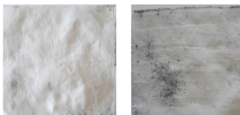
Figure 4. Tip ultrasound-assisted AgNPs deposition at 70% of ultrasound intensity using geometry B. Left sample: without plasma treatment. Right sample: with plasma treatment.
