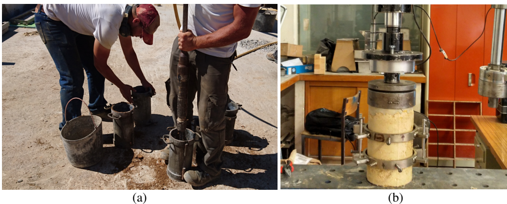
365 Fig. 9 – Compression tests: (a) sampling of the rammed earth specimens; (b) test setup.
