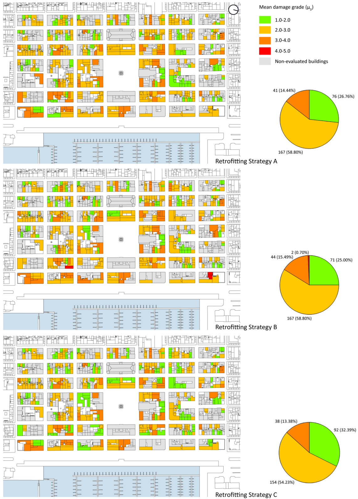
Figure 8.40: Damage scenarios for an earthquake with PGA = 0.25g considering the three retrofitting strategies
