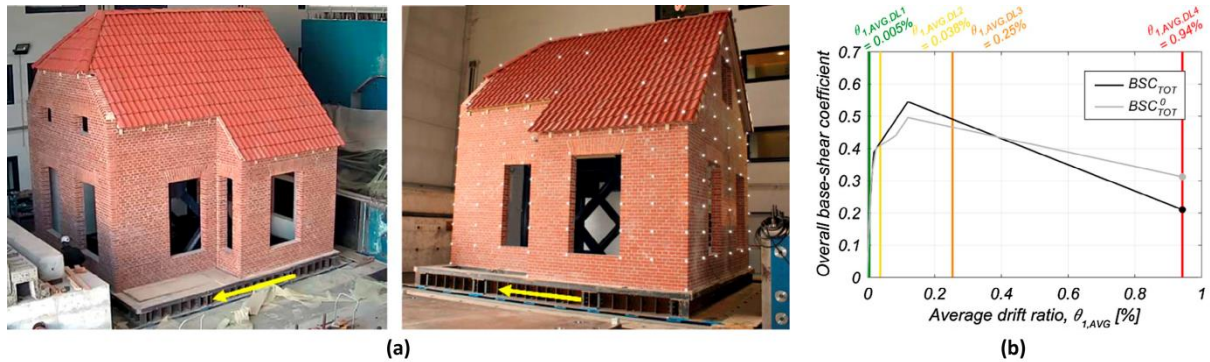
Figure 6.14: (a) Two-story full-scale building prototype; (b) overall building response in terms of base shear coefficients ( BSC ) versus drift (Kallioras et al. 2018)
