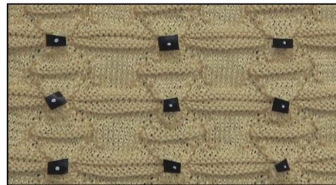
Fig. 7 Marked points in the fabrics to measure the distance between them
