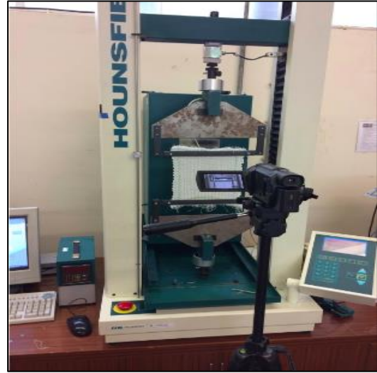
Fig. 6 Setup of testing Poisson's ratio
