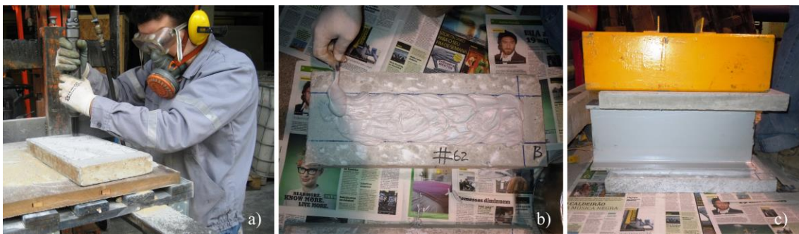
Figure 2 – Specimen preparation: a) roughening of the SFRSCC surface; b) application of the epoxy adhesive; and c) final aspect of the specimens.
