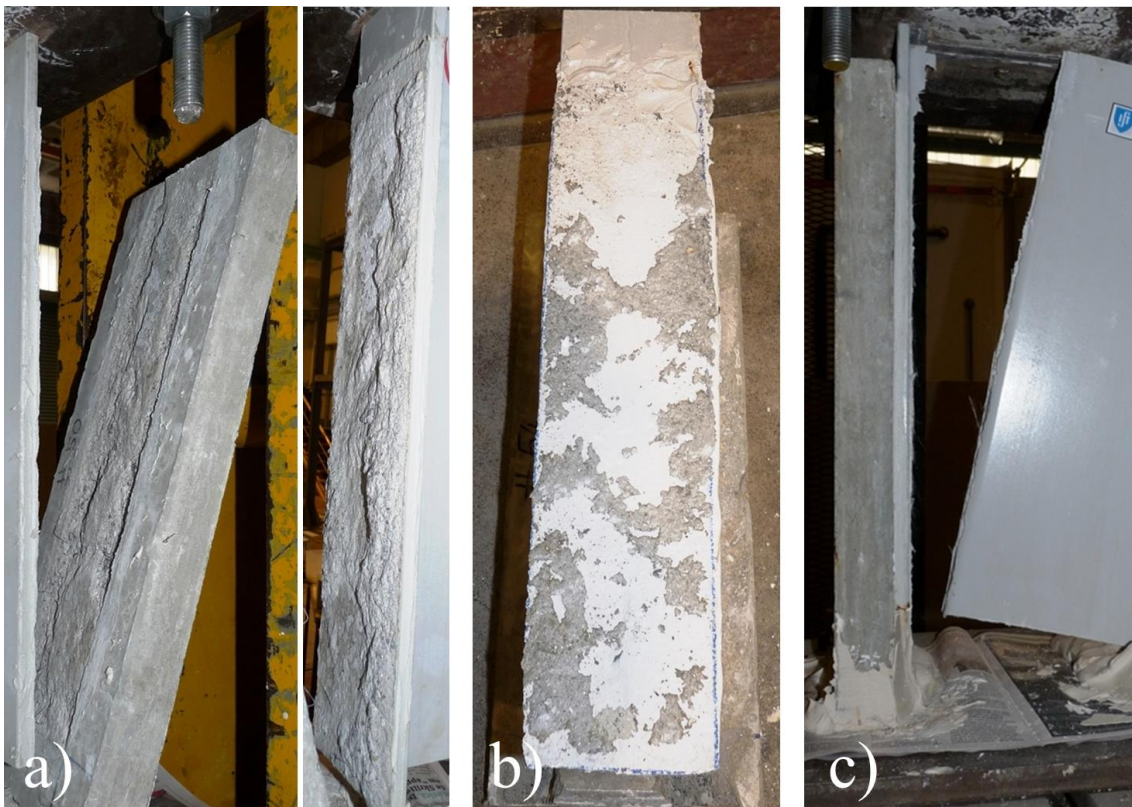
Figure 7 – Typical failure modes: a) debonding on the SFRSCC (cohesive failure); b) debonding on the epoxy (adhesive failure); and c) web-flange junction rupture.
