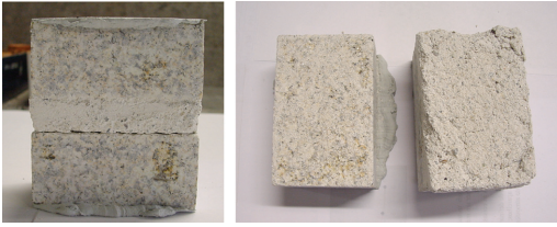
Figure 6. Typical Failure mode for the lower compression level ( \sigma = 0.5 \text{ N/mm}^2 ).
