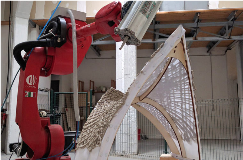
Figura 2.10. Tests made with Comau NJ60 6 axis robotic arm, Co.de.iT, 2018.
