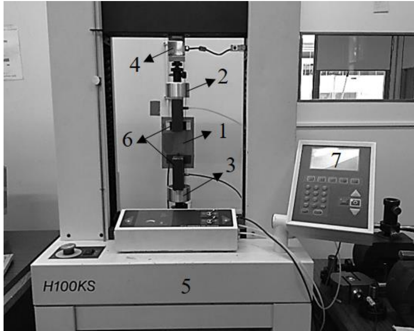
Figure 3.14. Dynamometer cyclic tester Hounsfield tester H100KS and the tensile test set based on ASTM D5034, grab test (1- Textile sample; 2- Dynamic cross head; 3- fixed cross head 4- Strain gauge loadcell; 5- Drive unit; 6- Wedge grips; 7- Digital display)
