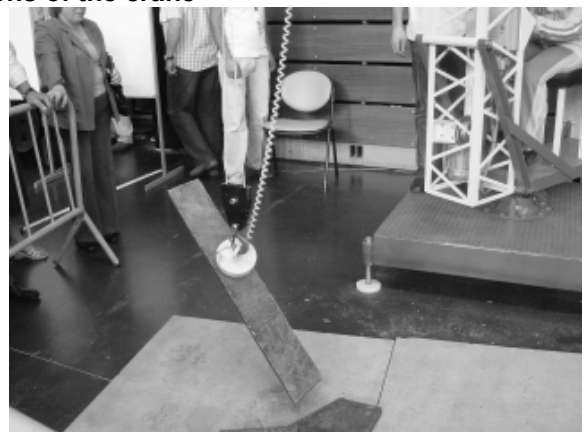
Figure 6. Electromagnet elevating an iron piece
