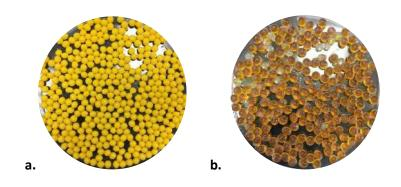
**Figure 1.** Beads of formulation A (**a**) and core-shell capsules of formulation F (**b**) produced using the Buchi Encapsulator B-395 Pro.
