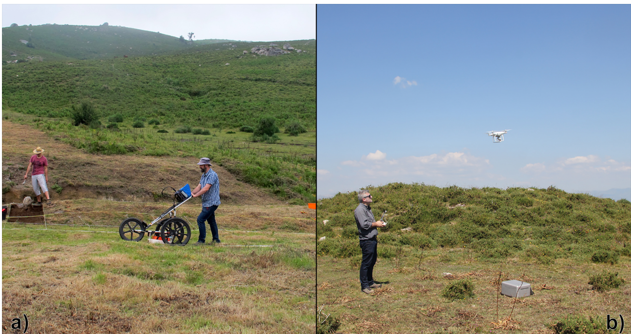
Fig.1. a) Geophysical prospection with GPR. b) Use of UAV for photogrammetry.
