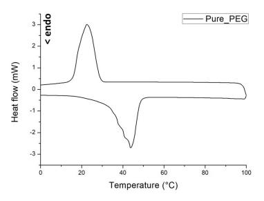
Figure 4. DSC thermograms recorded of pure PEG.
