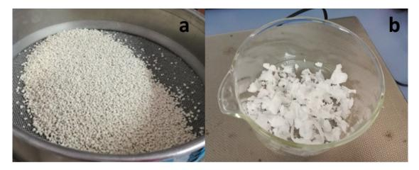
Figure 1. (a) Milled and sieved Lecce stone and (b) PEG 1000 in solid form.
