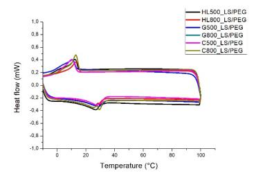
Figure 5. DSC thermograms of mortars containing LS/PEG PCM.
