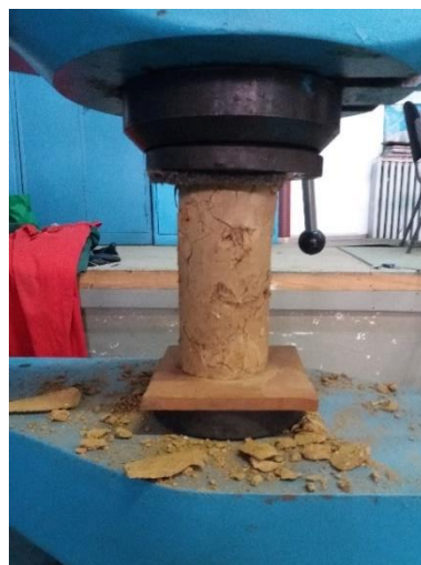
Figure 3.7 Compression test on mud cylinders (Dutu 2017).
