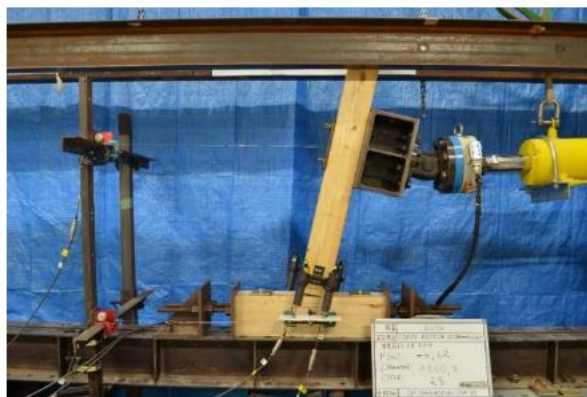
Figure 4.16 Test setup of CH connection (Dutu 2017).
