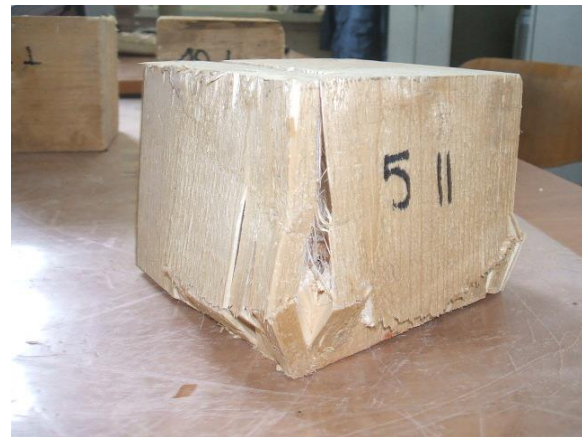
Figure 3.8 Damages on timber specimens after compression test parallel to fiber direction (Dutu 2017).
