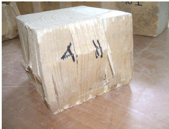
Figure 3.8 Damages on timber specimens after compression test parallel to fiber direction (Dutu 2017).
