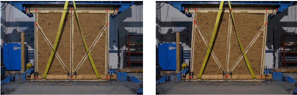
Figure 5.16 Undeformed (a) and deformed (b) shape just under vertical loads.
