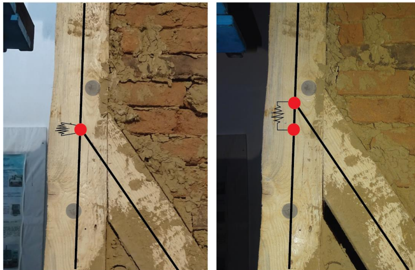
Figure 5.18 Vertical sliding along the post: initial and final position.
