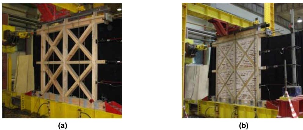
Figure 2.14 Tested walls: timber-framed wall (a), timber-framed masonry wall (b) (Gonçalves et al. 2012).
