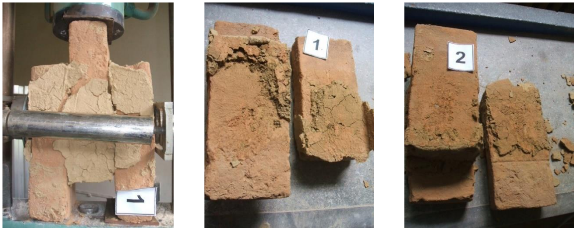
Figure 3.6 Shear test on masonry specimen (Dutu 2017).
