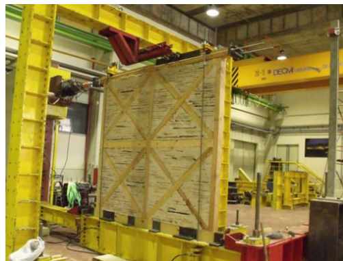
Figure 2.12 Pombalino “frontal” wall (Meireles et al. 2012).
