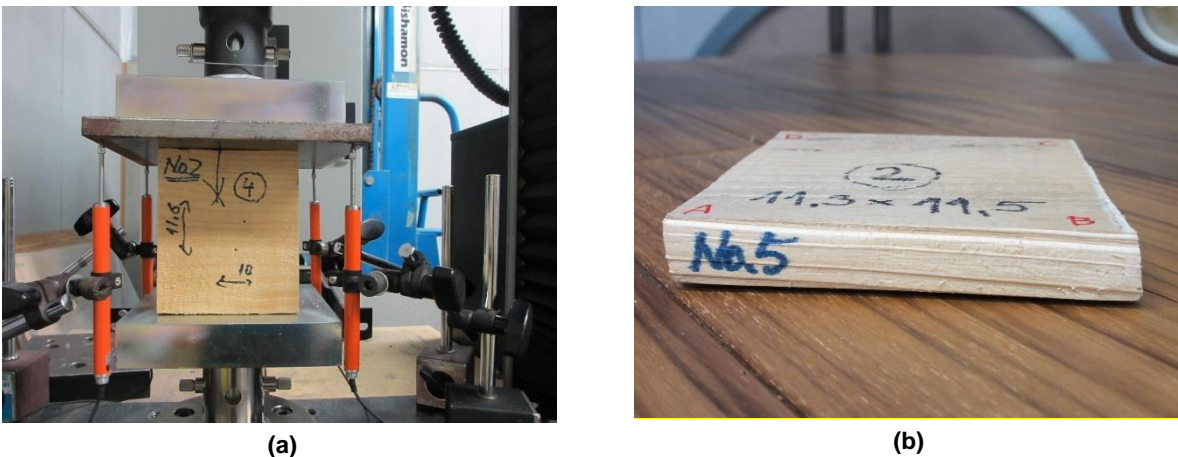
Figure 3.10 Compressive tests on timber specimens: cubic (a) and rectangular (b) (Dutu 2017).
