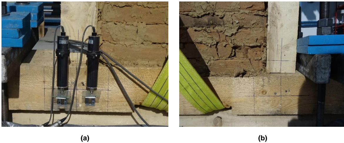
Figure 5.4 External post uplift (a) and rotation (b).
