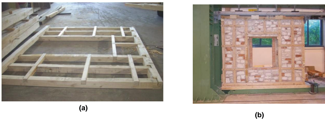
Figure 2.18 Timber frame (a) and tested wall (b) (Ruggieri 2015).
