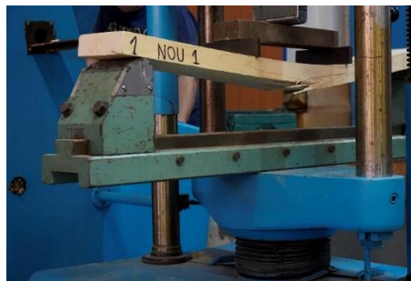
Figure 3.13 Four-point bending test on timber specimen.
