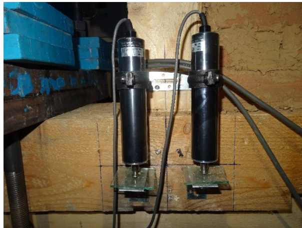
Figure 5.8 Negligible sliding between post and lower beam.
