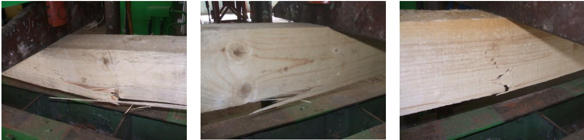
Figure 3.12 Types of failure mechanisms of 3-point bending test (Dutu 2017).
