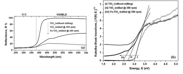
**Figure 2.** Diffuse reflectance spectroscopy of  $TiO_2$  nanoparticles (**a**) and calculation of the  $TiO_2$  energy band gap by the Kubelka–Munk theory (**b**). Reprinted with permission from [42]. Copyright 2014 Springer.
