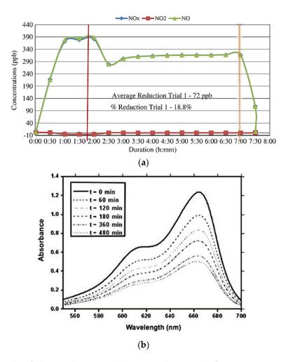
**Figure 5.** Results of photocatalytic tests: (**a**) variation (over time) of gas concentration, indicating its photodegradation (Reprinted with permission from [60] Copyright 2014 American Society of Civil Engineers); (**b**) absorbance variation (over time) of the dye's aqueous solution, indicating its photodegradation (Reprinted with permission from [6] Copyright 2013 Elsevier).
