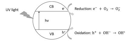
**Figure 1.** Schematic representation of the photo-excitation in a semiconductor material. Adapted with permission from [35]. Copyright 2003 Elsevier.
