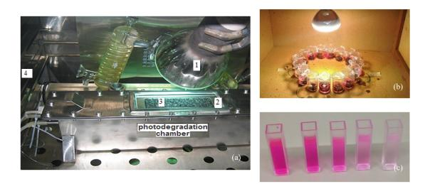
**Figure 4.** Experimental tests to measure the photocatalytic activity: (**a**)  $NO_x$  degradation efficiency (1: lamp for light irradiation, 2: quartz window, 3: test specimen, and 4: temperature stabilizer); (**b**) degradation of an organic dye; (**c**) aqueous solution of an organic dye of different color intensity over time, thus indicating its degradation.
