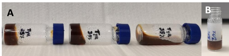
FIGURE 49. HYDROGEL AFTER THE HYPERTHERMIA ANALYSIS. A- MAGNETIC HYDROGEL 1 WITH INCORPORATED 25 %, 30% AND 35% OF SPIONS; B- MAGNETIC HYDROGEL 2 WITH INCORPORATED 30% SPIONS.
