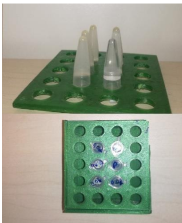
FIGURE 45. PICTURE OF SELF-ASSEMBLED HYDROGELS CONTAINING SPIONs (0-0.06% (M/M)) FOR MRI MEASUREMENTS.
