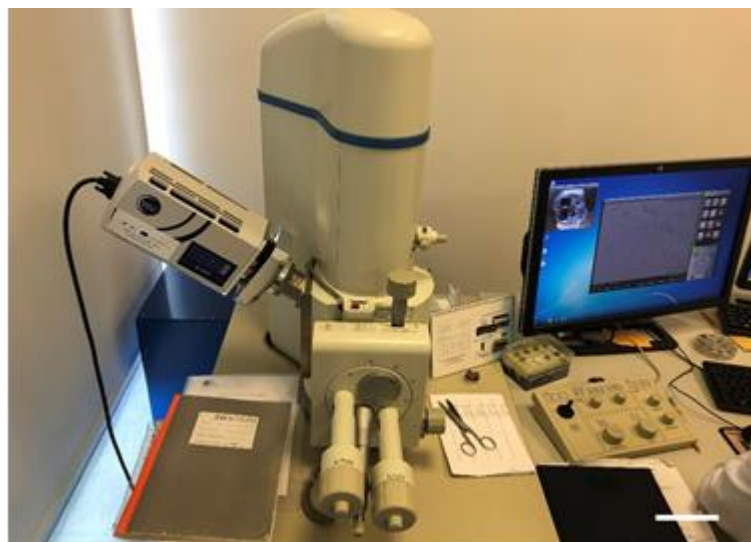
Figure IV-16 - SEM with EDS analyzer. The SEM (JSM-6010 LV, JEOL, Japan) instrument is equipped with the low vacuum mode as a standard feature. The low vacuum mode allows non-conductive specimens to be observed and analyzed without conductive coating. This SEM is equipped with an energy dispersive spectroscope (EDS). Scale bar: 10 cm.
