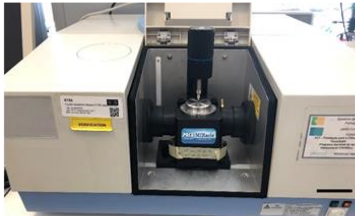
Figure IV-17 - The Fourier transform infrared (FTIR) spectrometer is used as a standard chemical characterization technique. The samples can be analyzed as films, KBr discs, powder or liquids. The available methodologies comprise transmittance, specular reflectance, diffuse reflectance and attenuated total reflectance (ATR). Scale bar: 10 cm.
