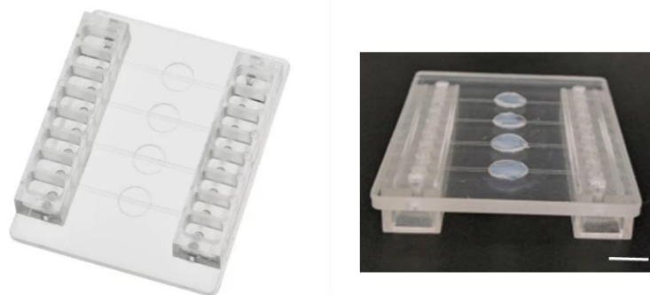
Figure IV-10 – Vena4™ empty and with silk hydrogels placed on the microwells. Scale bar: 6 mm.
