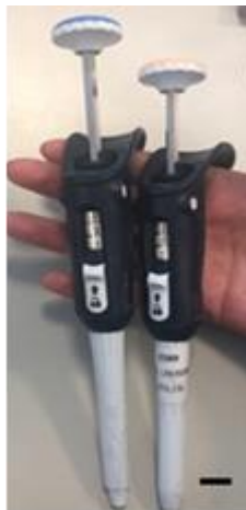
Figure IV-9 - Micropipettes Gilson M100 and M1000, specifically designed for hydrogel use. Scale bar: 1 cm.
