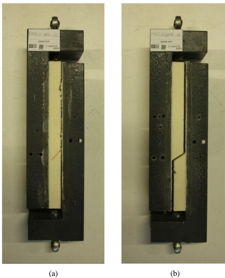
642 Figure 5 - Failure modes identified in the tests performed to assess shear strength of the PIR foam: (a) FM1 - 643 shear crack parallel to the steel plates; (b) FM2 - transverse shear crack.
