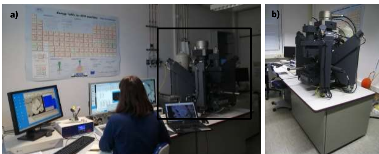
Figure 28 – Electron microprobe. a) Image of the general equipment required for electron microprobe use. b) Detail for the Cameca SX100 electron microprobe (from “Electron probe microanalysis” in https://www.ozeankruste.uni-bremen.de/index.php/en/laboratories/electronmicroprobe.html ; accessed on 24 th of June of 2019).
