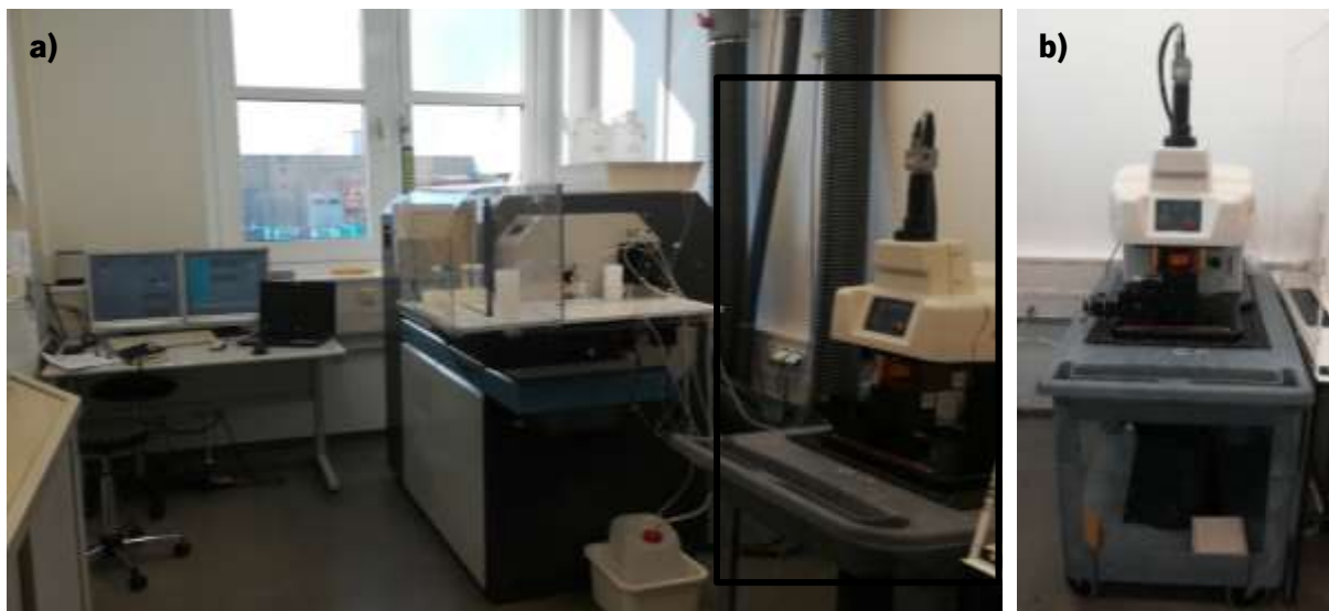
Figure 29 – Laser-ablation inductively coupled plasma mass spectrometry. a) General image of the equipment required for laser-ablation inductively coupled plasma mass spectrometry use. b) Detail for the New Wave UP193 laser.
