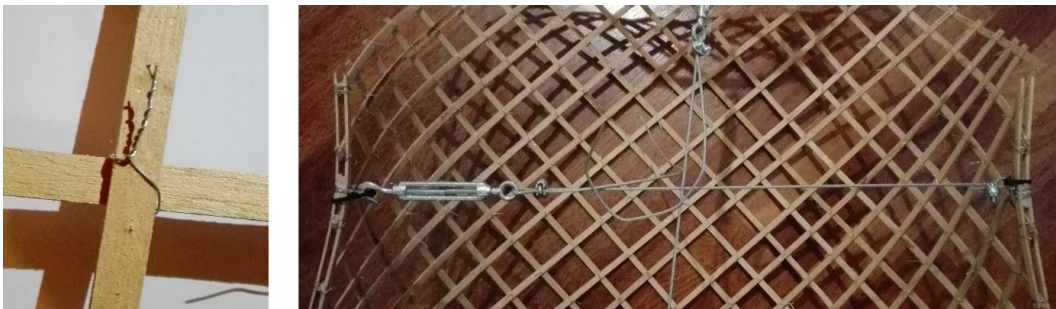
Figure 5.5- Final connection and cable system
