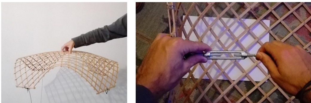
Figure 5.4- Lifting and tightening of the grid stiffeners
