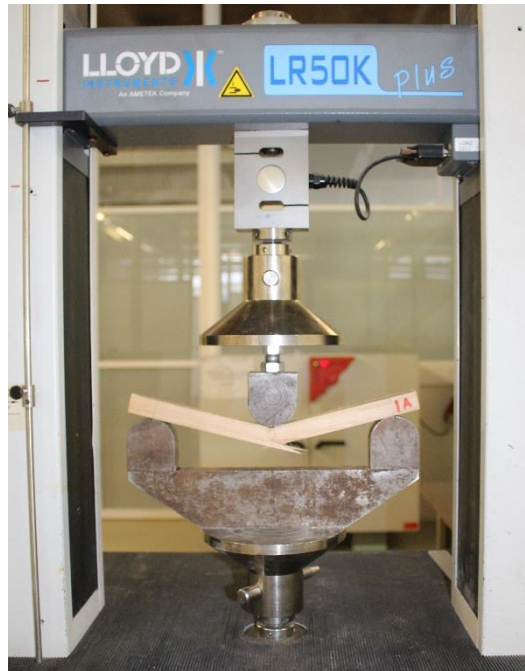
Figure 5.37- Bending test setup
