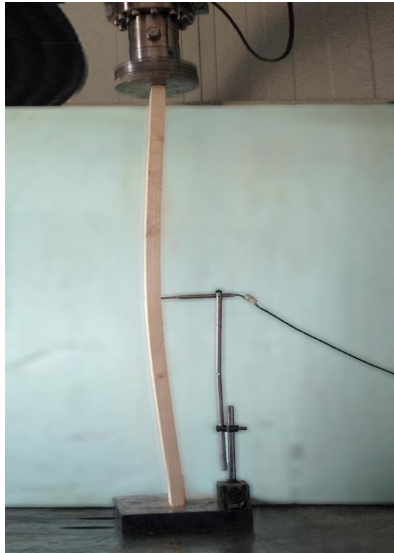
Figure 4.6- Buckling test scheme
