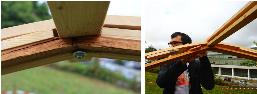
Figure 5.29- Breaking of two timber elements
