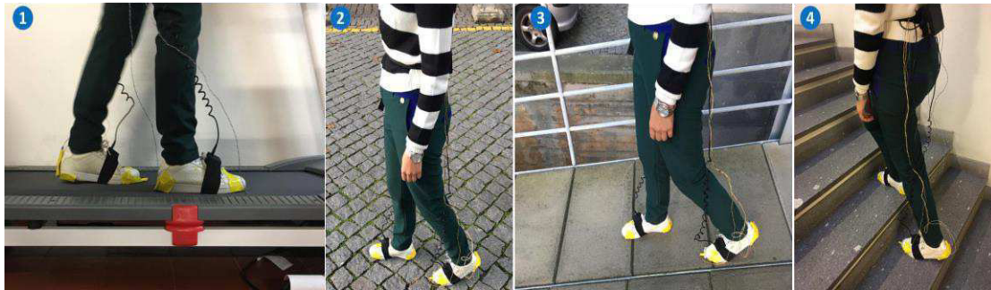
Figure 5.3- Validation of the gait event detection system under controlled (1) and real-life walking conditions (2- flat and rough level-ground, 3-ramp, 4-stairs). The users wore two IMUs of InertialLAB (instep of the foot) and two FSRs attached to heel and toe by a yellow rubber strap [52].
