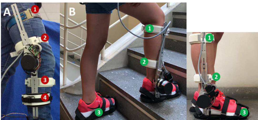
Figure 7.2- AOs' attachment system. A: Four-strap System (1-4). B: Two-strap System (1-2) and four-strap system built-in the PAFO's outsole (3).
