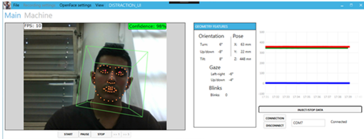
Figure 19 - The GUI displaying the webcam feed, the user's eye gaze and head pose (left), and the IMU values on a chart (right).
