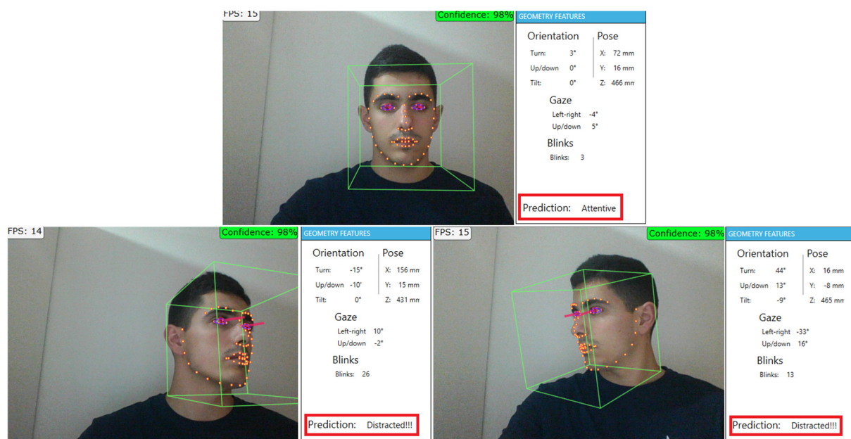
Figure 26 - The GUI displaying the classification considering different poses (results using Gaussian SVM method). The classifier output is presented in the interface (red rectangles).
