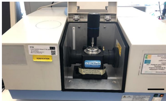
Figure IV-22 - The Fourier transform infrared (FTIR) spectrometer is used as a standard chemical characterization technique. The samples can be analyzed as films, KBr discs, powder or liquids. The available methodologies comprise transmittance, specular reflectance, diffuse reflectance and attenuated total reflectance (ATR). Scale bar: 10 cm.
