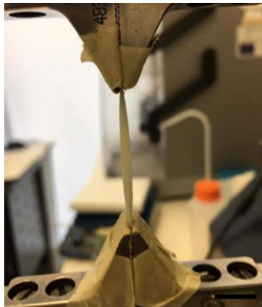
Figure IV-25 - Enzymatically crosslinked SF conduits being tested in tensile mode with Instron equipment. Scale bar: 10 mm.
