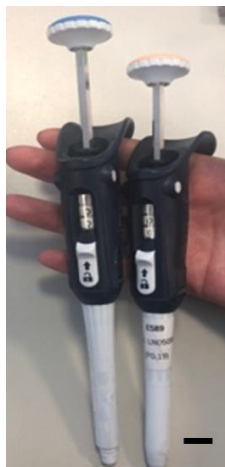
Figure IV-12 - Micropipettes Gilson M100 and M1000, specifically designed for hydrogel use. Scale bar: 1 cm.
