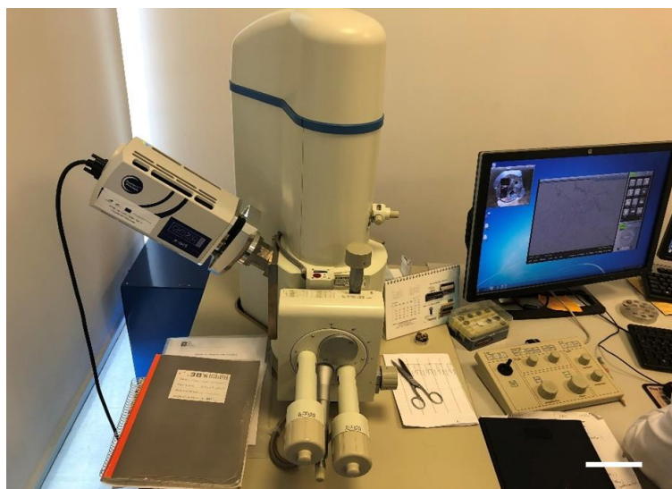
Figure IV-16 - SEM with EDS analyzer. The SEM (JSM-6010 LV, JEOL, Japan) instrument is equipped with the low vacuum mode as a standard feature. The low vacuum mode allows non-conductive specimens to be observed and analyzed without conductive coating. This SEM is equipped with an energy dispersive spectroscope (EDS). Scale bar: 10 cm.
