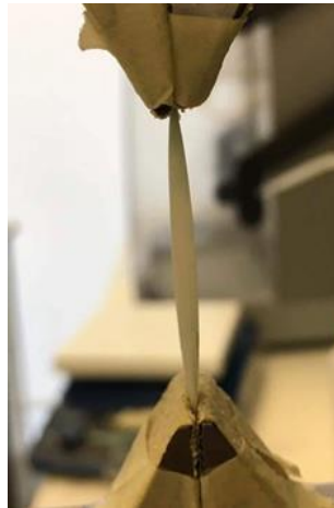
Supplementary Figure IX-4 - Apparatus used for universal mechanical testing machine (Instron) for tensile tests in the developed TCs. Both TC ends were hold with a grip.
