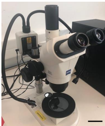
Figure IV-15 - Stereomicroscope from Zeiss, used for macroscopic evaluation of samples in this thesis. Scale bar: 5 cm.
