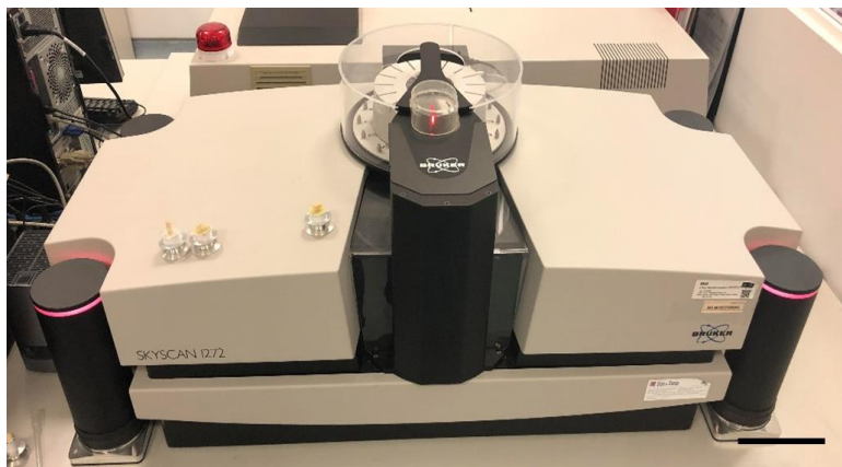
Figure IV-17 - Micro computed tomography for non-destructive 3D analysis of bulk structure of scaffolds. Output is the general structure as a 3D model with micrometer resolution, more importantly the subsequent analysis can yield information in relation to pore size, pore distribution and pore interconnectivity in 3D. Scale bar: 10 cm.
