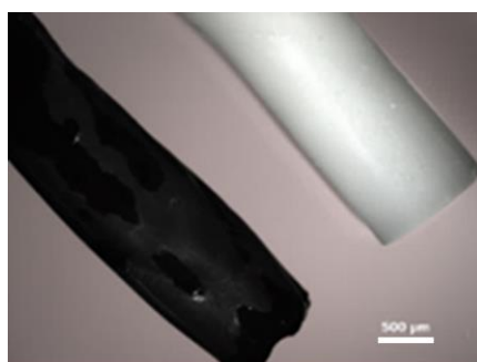
Figure VIII-9 - Schematic representation of a simple hydrated silk conduit (white) when compared to a conductive silk/polypyrrole conduit (black). Scale bar: 500 µm.
