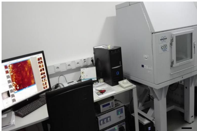
Figure IV-18 - The AFM is able to acquire images of flat surfaces that can encode the surface topography, mechanical response, among other properties. The equipment presents a series of accessories that allows the acquisition of data in liquids and air. In the case of liquids, it is also possible to control the temperature of the experiments. Scale bar: 10 cm.
