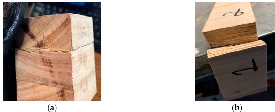
Figure 7. Typical wood shear failure observed during the shear tests performed. (a) Surface-bonding specimens (Bi) and (b) edge-bonding specimens (Ei).
