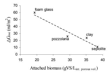
Figure 1 Relation between the attached anaerobic biomass and the degree of hydrophobicity of various inorganic carriers, expressed as  $\Delta G_{iwi}$ .
