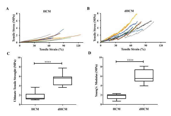
**Figure 3.** Mechanical properties of native and decellularized HCM. Stress-strain curves of HCM (**A**) and dHCM (**B**). Ultimate tensile strength (**C**) and Young's modulus (**D**) of both HCM and dHCM. \*\*\*\*  $p \le 0.0001$ .
