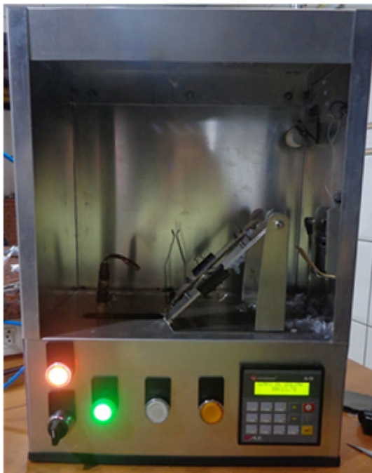
Fig. 3 Flammability test cabin built for the flame speed experiments
