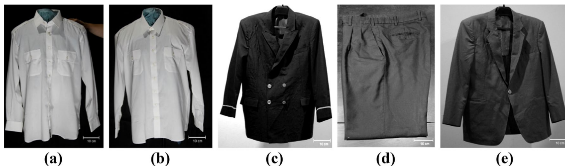
Fig. 2 Uniforms of Airline company “B”: a , b P4 and P5—67% PES/33% CO plain fabric male shirts; c P6—55% PES/45% WO male coat; d P7—50% PES/50% WO male trousers; e P8—55% PES/45% WO male coat
