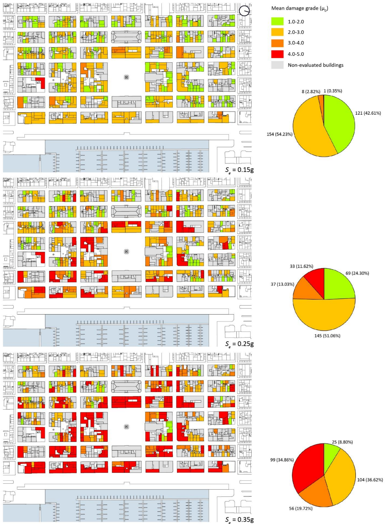
312 Figure 9. Damage scenarios for different seismic input in terms of seismic demand ( S_e ) : (a) 0.15g; (b) 0.25g; and 313 (c) 0.35g
