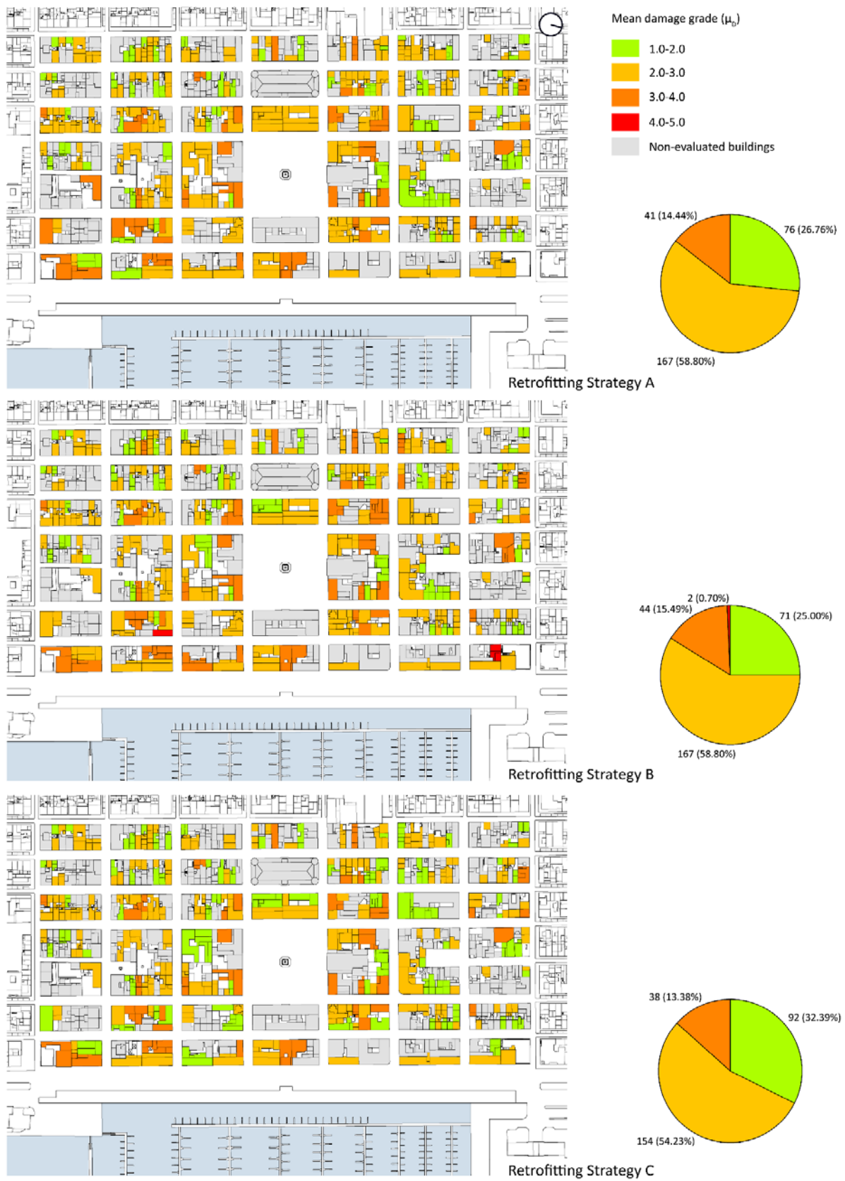
498 Figure 15. Damage scenarios for an earthquake with S_e = 0.25g ( PGA = 0.18g ) considering the three 499 retrofitting strategies
