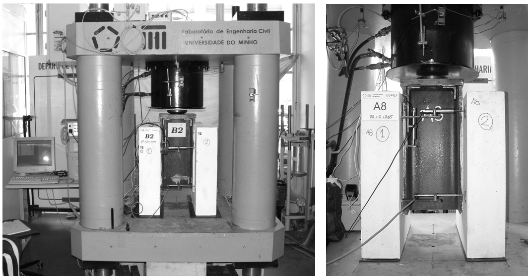
Figure 7 - Push-out test setup.
