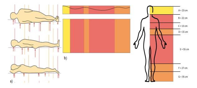
Figure 3. a) Illustrative diagram of the division of the pressure zones; b) segmentation and levels of body immersion.
