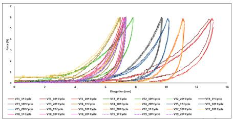
Figure 5. Absorbed energy measured in each sample (from VT\_1 to VT\_9) in the 1<sup>st</sup>, 10<sup>th</sup> and 20<sup>th</sup> cycles.
