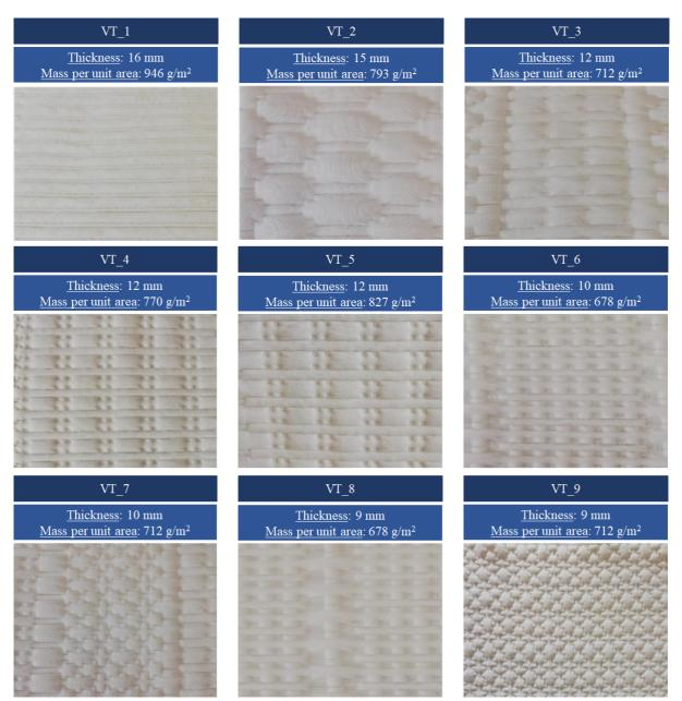
Figure 4. Patterns used in the methodology of the study of the surface design.
