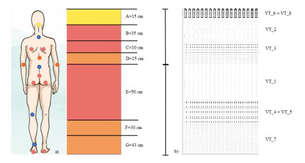
Figure 7. a) diagram on the body pressure points and mattress overlay; b) optimized overlay and sample identification.
