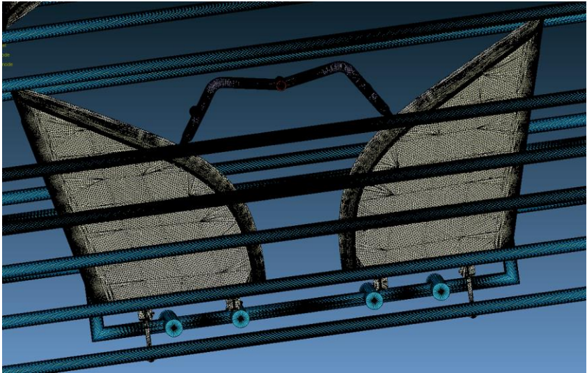
Figure 4.5 - Zoomed view of the mesh generated.
