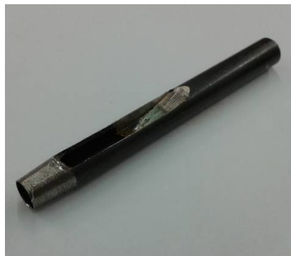
Figure 24: Standard hollow-punch for cylinder-shaped samples.
