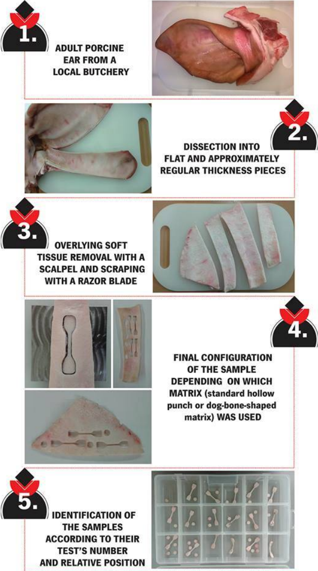
Figure 26: A procedure for porcine auricular cartilage samples preparation.
