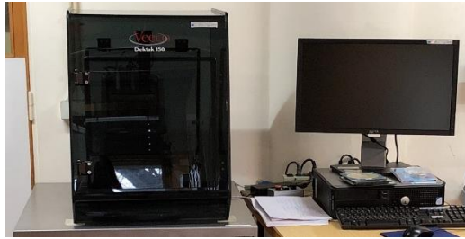
Figure 39. Experimental setup for roughness measurements.
