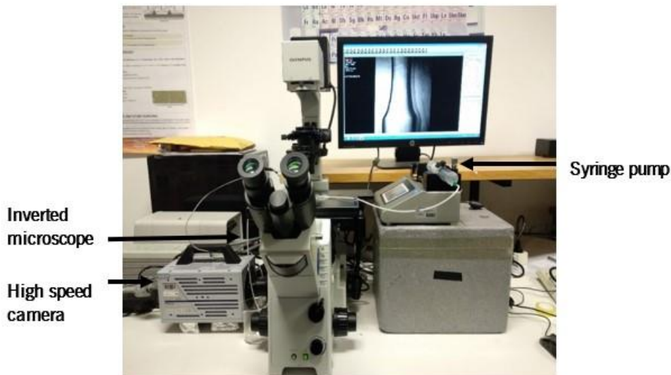
Figure 40. Experimental setup used to control and visualize the flow.
