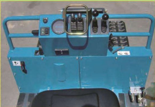
Details of the dashboard with controls and hydraulic P.T.O. Detail Instrumentenbrett und Nebenantrieb
