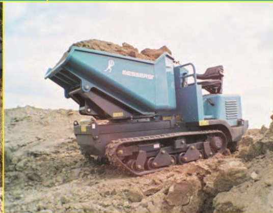
180° TCH-1500/BT swivelling skip during working phases / TCH-1500/BT mit 180° Drehmulde in Arbeitsphase /
