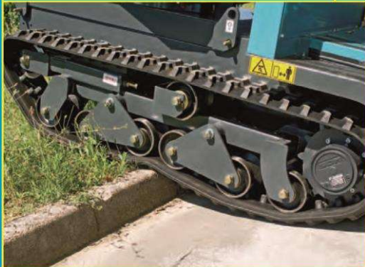
Details of the track swing / Detail Raupenschwung /
