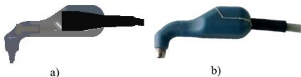
Figure 2. Prototype tool for implant acquisition; a) cross section; b) final assemble.
