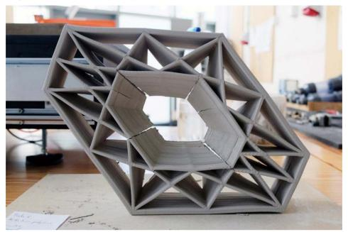
Figure 5. Hexashade, test arch 1 – real scale – interior wall break.
