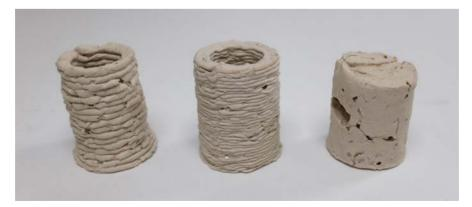
Figure 6: Tests of ceramic paste with fiberglass (5%).
