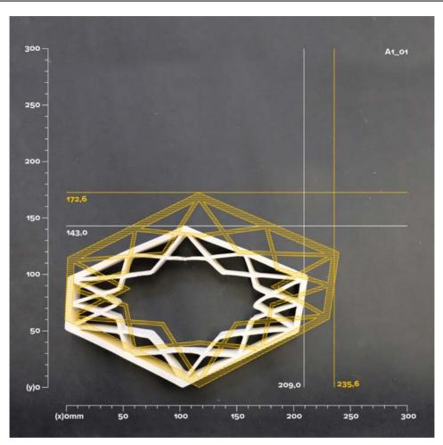
Figure 4. Hexashade, test arch 1 – piece 1 – retraction analysis.
