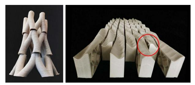
Figure 1. Segmented Ficus column - Initial test. Wave Wall - Effects of friction in retraction.
