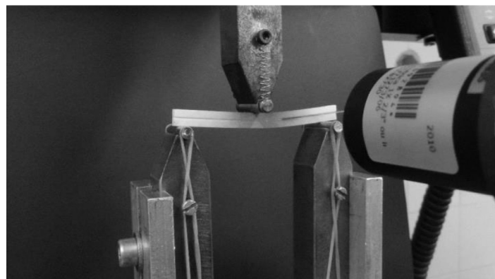
Fig. 2. Testing setup of the ENF test showing the speckle pattern.
