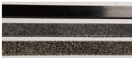
Figure 1. Surface configuration of CFRP laminates: (top) untreated, (middle) treated with Carga2 (bottom) treated with fine sand
