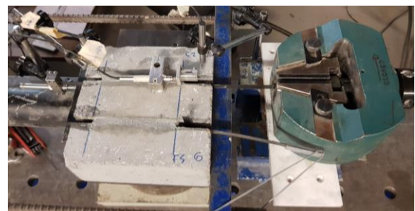
Figure 4. Photo of pull-out tests with NSM CFRP laminates
