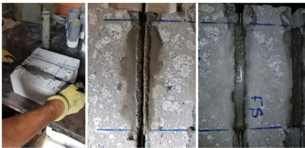
Figure 3. Process of introducing CFRP laminates into the grooves from left to right
