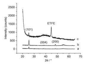
**Figure 15.** XRD patterns of anatase TiO<sub>2</sub> films in substrates made of (**a**) Si at 200 °C, (**b**) PMMA at 250 °C, and (**c**) ETFE at 200 °C. Si substrate was used as a reference, for comparison purpose (reprinted from [66] Copyright (2008), with permission from Elsevier).
