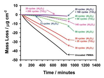
**Figure 14.** Mass loss of uncoated and coated PMMA with Al<sub>2</sub>O<sub>3</sub> and Al<sub>2</sub>O<sub>3</sub>/TiO<sub>2</sub> when exposed to vacuum UV radiation over time (reprinted with permission from [65], Copyright (2010) American Chemical Society).
