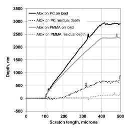
**Figure 7.** On-load and residual depth curves for Al<sub>2</sub>O<sub>3</sub>/PMMA and Al<sub>2</sub>O<sub>3</sub>/PC (polycarbonate) after the nanoscratch. The test was repeated five times per sample; each scratch had 500  $\mu$ m of length, at a scanning velocity of 10  $\mu$ m/s, and a ramped load varying from 0.1 mn to 60 mn (reprinted with permission from [53], Copyright 2012, American Vacuum Society).
