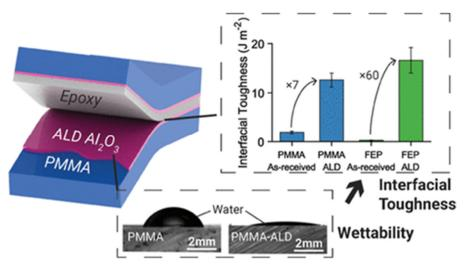
**Figure 8.** Thermoplastic-epoxy resin with the double Al<sub>2</sub>O<sub>3</sub> coating; wettability test of a water droplet in coated and uncoated PMMA surface, and the interfacial toughness of PMMA and fluorinated ethylene propylene (FED) (wedge test) (reprinted with permission from [54], Copyright (2019), American Chemical Society).
