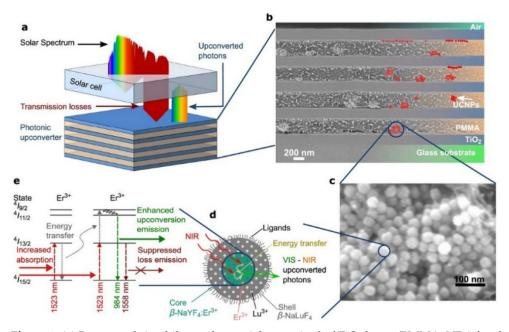
**Figure 9.** (a) Bragg stack (multilayered material comprised of TiO<sub>2</sub> layers/PMMA+NPs) for charge generation in a solar cell by a photonic upconverter. SEM image of the (b) Bragg stack and (c) of
