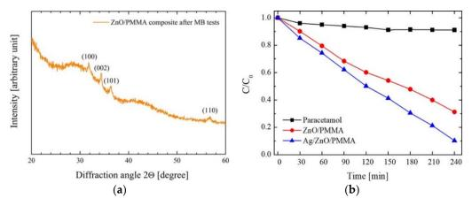
**Figure 11.** XRD pattern of ZnO/PMMA composite after the seven MB discoloration runs [62]. (a) Degradation of paracetamol drug as a function of irradiation time for paracetamol alone (squares), paracetamol with ZnO/PMMA (circles), and paracetamol with Ag/ZnO/PMMA (triangles) samples (b), under UV illumination [61] [both works by Alessandro Di Mauro are licensed under a Creative Commons Attribution (CC BY 4.0).
