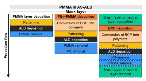
**Figure 21.** PMMA in an AS-ALD process, where the block copolymers are polystyrene-*random*-poly(methylmethacrylate) (PS-*r*-PMMA) or polystyrene-*block*-poly(methylmethacrylate) (PS-*b*-PMMA).
