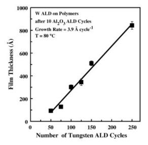
**Figure 13.** Profilometry measurements of W ALD film thickness on different polymers vs. the number of W ALD cycles. Al<sub>2</sub>O<sub>3</sub> ALD was used as a seed layer (10 ALD cycles) (reprinted from [64], Copyright (2008), with permission from Elsevier).
