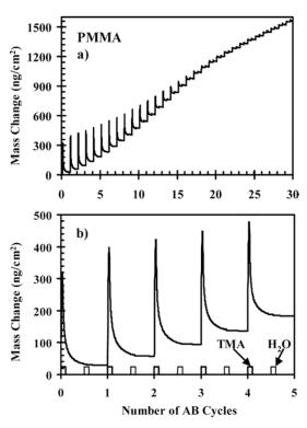
**Figure 5.** Mass change measurements by QCM versus number cycles of Al<sub>2</sub>O<sub>3</sub> ALD on PMMA at 85 °C for (a) 30 and (b) 5 cycles (reprinted with permission from [40], Copyright (2005) American Chemical Society).
