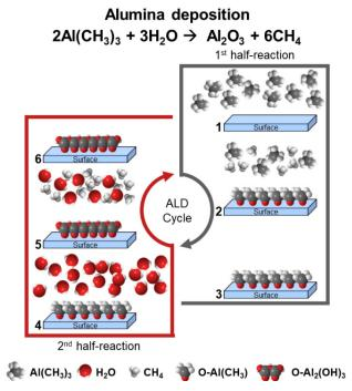
**Figure 2.** Schematic representation of the ALD formation of the first Al<sub>2</sub>O<sub>3</sub> monolayer from: (1) TMA pulsing; (2) TMA chemisorption in the surface (first half-reaction); (3) after purging of unreacted TMA and methane; (4) water pulsing; (5) water chemisorption on the by-product from the first half-reaction; and (6) after purging of unreacted water and methane.
