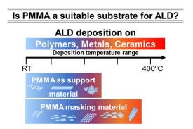
**Figure 1.** Schematic illustration of ALD application range: deposition temperature and types of substrates. The ability to perform ALD at low temperatures is well suitable to deal with thermally sensitive materials such as PMMA. As a support material, PMMA can be produced such as thick plates, spin-coated films, powder, nanoparticles, amongst other forms.
