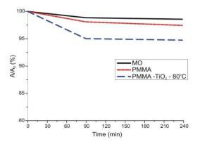
**Figure 10.** Photocatalytic efficiency of the amorphous TiO2. After 90 min, the methylene orange dye degraded 5% under UV-A illumination [adapted from [59], this work by Orsolya Kéri is licensed under a Creative Commons Attribution (CC BY 4.0)].
