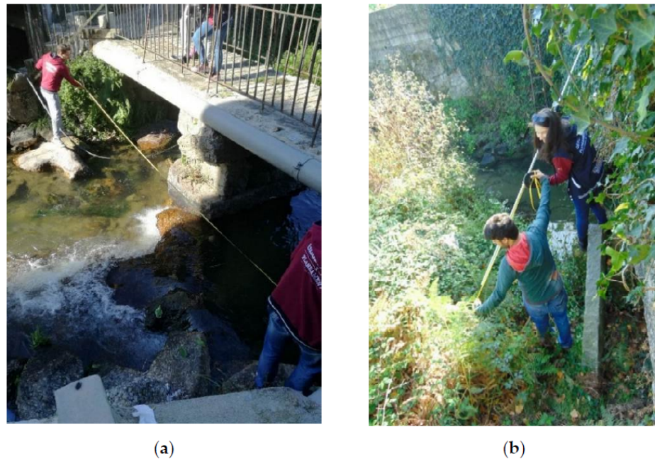
Figure 8. Channel surveying, associated with Section L: (a) width measurements; (b) height measurement.
