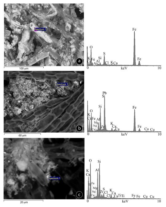
**Figure 6.** SEM (ES) micrographs and EDS analysis showing the relation between acidophilic algae and iron oxyhydroxides and hydroxysulfates. (a) Interconnection between algal filaments and iron cylindrical tubes; (b) multicellular and unicellular algae in the sediment; (c) Intergrowth morphology of *Pinnularia sp.* in sediment bearing Si and Al.
