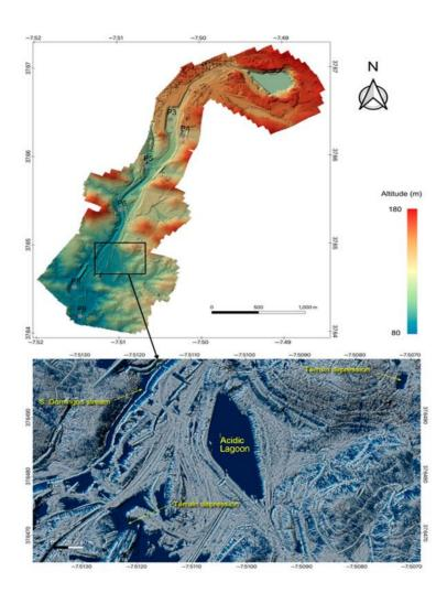
**Figure 3.** Digital Surface Model of the surveyed area obtained by UAV (**upper**); Section of the flow accumulation map (**lower image**) in the area with the finest sulfide wastes. In the lower part of the figure, the blue lines are flow lines of surface runoff and the blue continuous zones are areas of flow accumulation. Coordinates in WGS 84.
