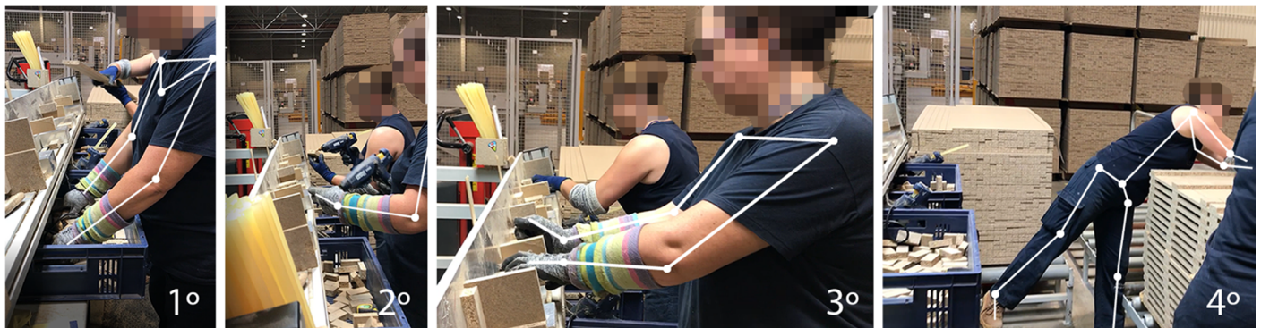
Figure 3. Workers postures during the assembly work cycle.
