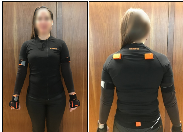
Figure 5. Participant with the 11 inertial sensors attached.
