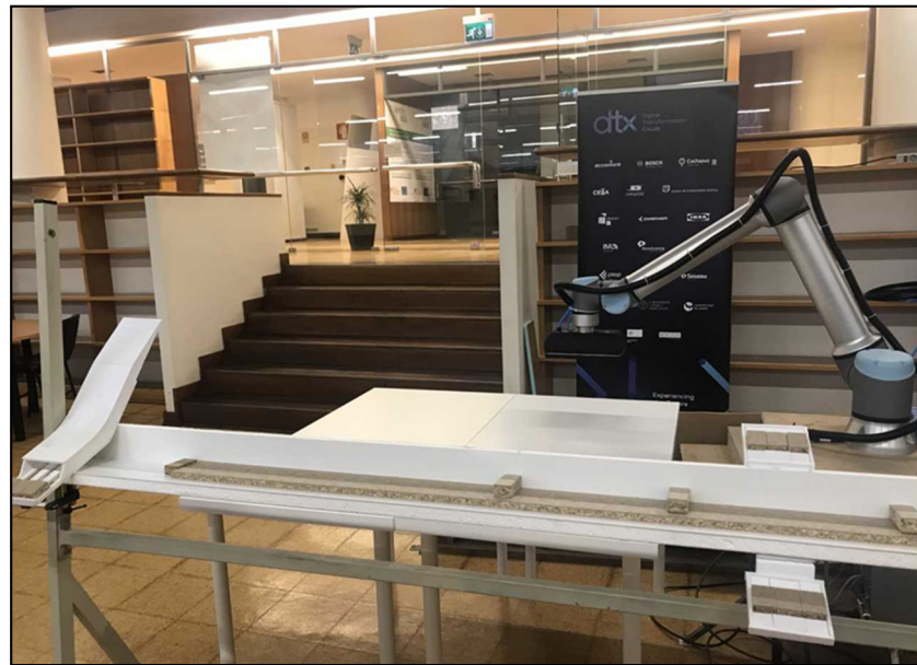
Figure 9. The prototype of the hybrid assembly workstation.
