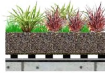
Semi intensive green roof
