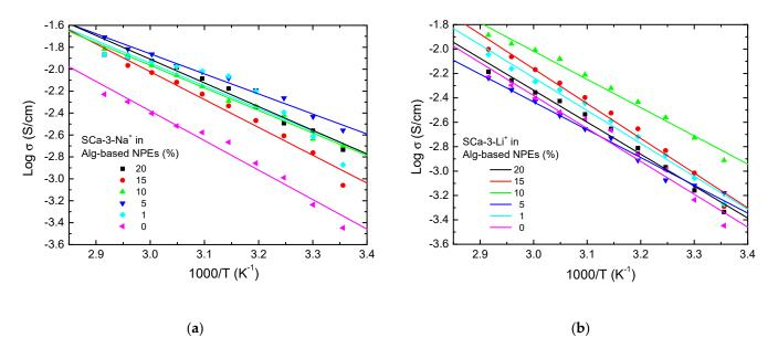
**Figure 5.** Log of conductivity in function of temperature for Alg-based NPEs with 0–20 wt% of (**a**) SCa-3-Na<sup>+</sup> and (**b**) SCa-3-Li<sup>+</sup>.
