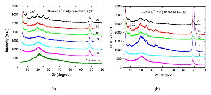
**Figure 1.** XRD for alginate powder, SCa-3-Na<sup>+</sup>, SCa-3-Li<sup>+</sup> clays, and Alg-based NPEs with 0–20 wt% of (**a**) SCa-3-Na<sup>+</sup> and (**b**) SCa-3-Li<sup>+</sup>.
