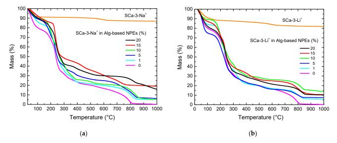
**Figure 2.** Thermograms for SCa-3-Na<sup>+</sup> and SCa-3-Li<sup>+</sup> clays and Alg-based NPEs with 0–20 wt% of (**a**) SCa-3-Na<sup>+</sup> and (**b**) SCa-3-Li<sup>+</sup>.
