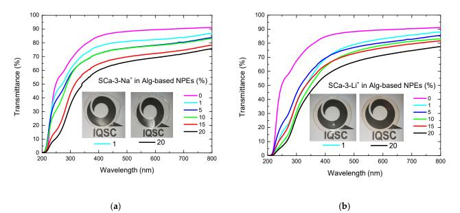
**Figure 3.** Transmittance spectra for Alg-based NPEs with 0–20 wt% of (**a**) SCa-3-Na<sup>+</sup> and (**b**) SCa-3-Li<sup>+</sup>. Inset photos of Alg-based NPEs with 1 and 20 wt% of clay.
