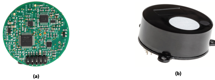
Figure 3.6: CozIR-A CO2 Sensor
