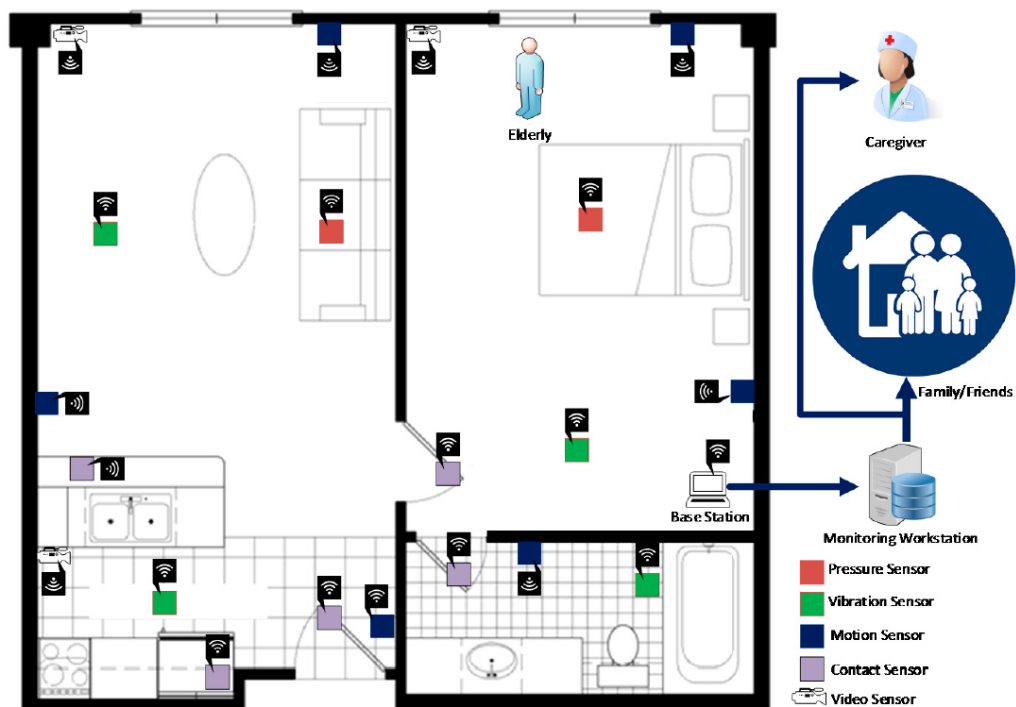
Figure 2.1: Schematic setup for elderly care based on different sensing technologies
