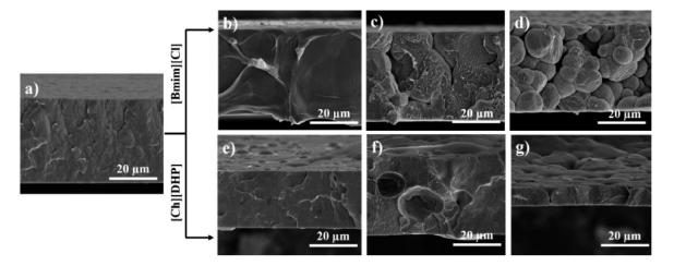
**Figure 7.** Cross section SEM images of (**a**) PVDF pristine and composite films with (**b**) 10% wt. [Bmim][Cl], (**c**) 20% wt. [Bmim][Cl], (**d**) 40 wt% [Bmim][Cl], (**e**) 10 wt% [Ch][DHP], (**f**) 20 wt% [Ch][DHP], and (**g**) 40 wt% [Ch][DHP]. Reprinted with permission from [114].
