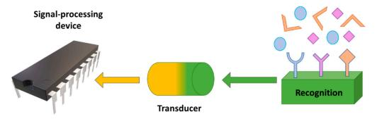
Figure 18. Schematic representation of the main elements of a generic biosensor.
