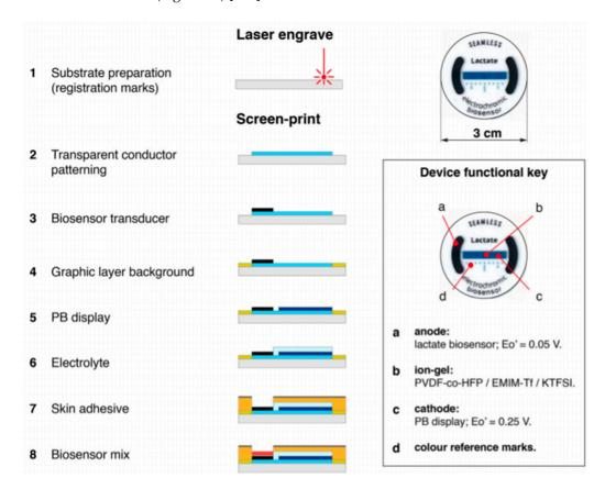
**Figure 21.** Diagrammatic representation of the fabrication process and photographs from two different prototype versions. The inset highlights the function of the device various components. Reprinted with permission from [210].
