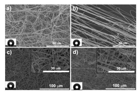
**Figure 8.** Morphology of electrospun polymer fiber mats: (**a**) randomly oriented neat PVDF, (**b**) aligned neat PVDF fibers, (**c**) randomly oriented PVDF with 5 wt% IL, and (**d**) aligned PVDF fibers with 5 wt% IL [Emim][TFSI] obtained. Reprinted with permission of [117].
