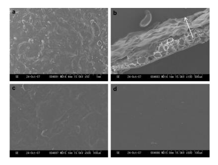
**Figure 5.** SEM micrographs of  $\alpha$ -chitin samples obtained with [Bmim][Ac] as solvent: (**a**) surface and (**b**) cross-section of freeze-dried sponge, (**c**) surface of oven-dried film with methanol as anti-solvent, and (**d**) surface structure of oven-dried film with water as anti-solvent. Reprinted with permission from [78].
