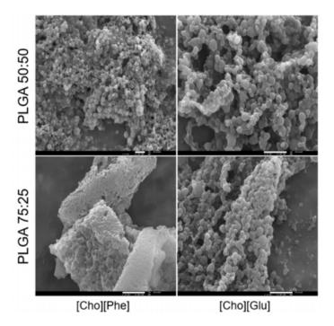
**Figure 6.** SEM micrographs of rutin-loaded IL-polymer nanoparticle hybrid systems after freeze drying at a magnification of  $4000 \times$  (PLGA 50:50/[Cho][Phe] and  $10,000 \times$  (remaining images). The scale bar of the micrographs at the bottom right of the images corresponds to 2 µm. Reprinted with permission from [114].
