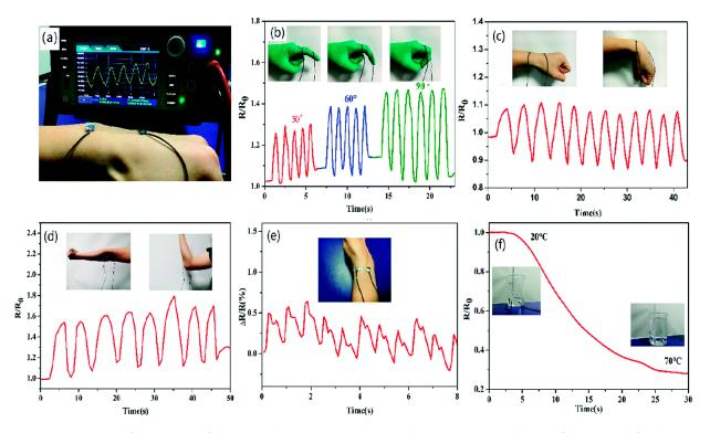
**Figure 19.** (a) Image of the testing of the ionogel strain sensor. (b–d) Relative resistance change of the ionogel for detecting different human motion: bending and straightening of the index finger, the wrist, and the elbow. (e) Relative resistance change of the ionogel for monitoring the beating of the human pulse. (f) Relative resistance change of the ionogel for monitoring the temperature change. Reprinted with permission from [204].
